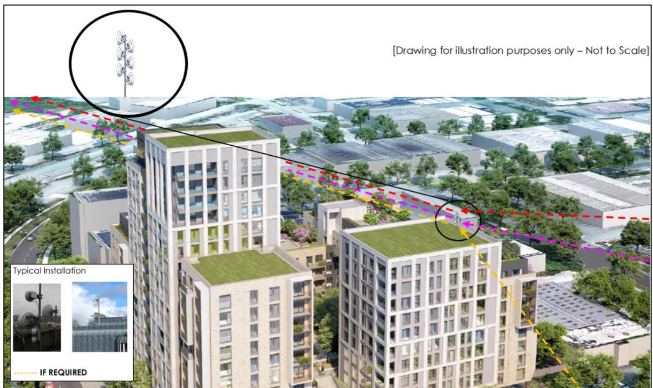
Figure 14.6: Microwave Links surrounding the Carmanhall Road SHD (ISM Limited 2021).
